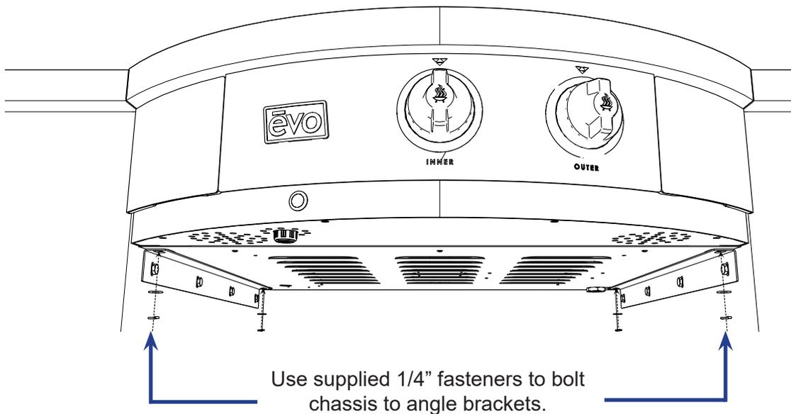
**STEP 4:** Slide the Affinity 30G chassis into the counter top so it rests on top of the installed brackets. Bolt unit to angle brackets using supplied 1/4" x 20 fasteners from underside.
