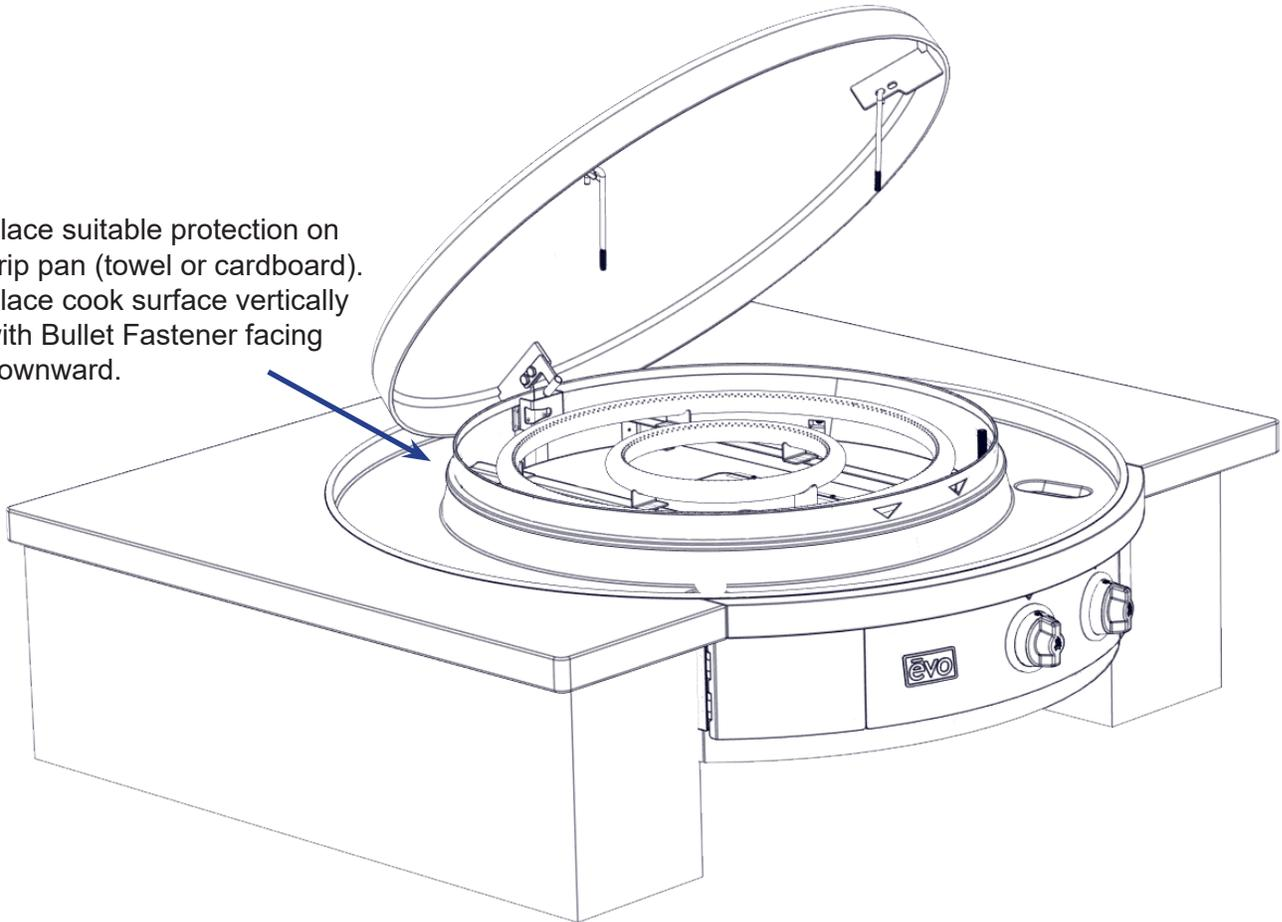
**STEP 8:** Position the cook surface at the rear of the burner chassis by placing the cook surface in the area of the drip pan, separated by a towel or cardboard to prevent damage to the drip pan.
