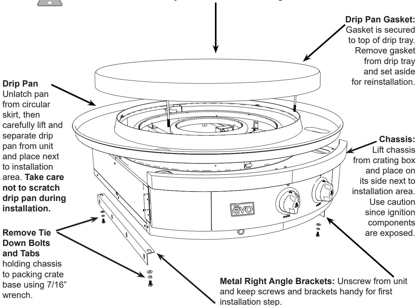
**STEP 1:** As you are unpacking the crate, make sure you locate all components before installation.
