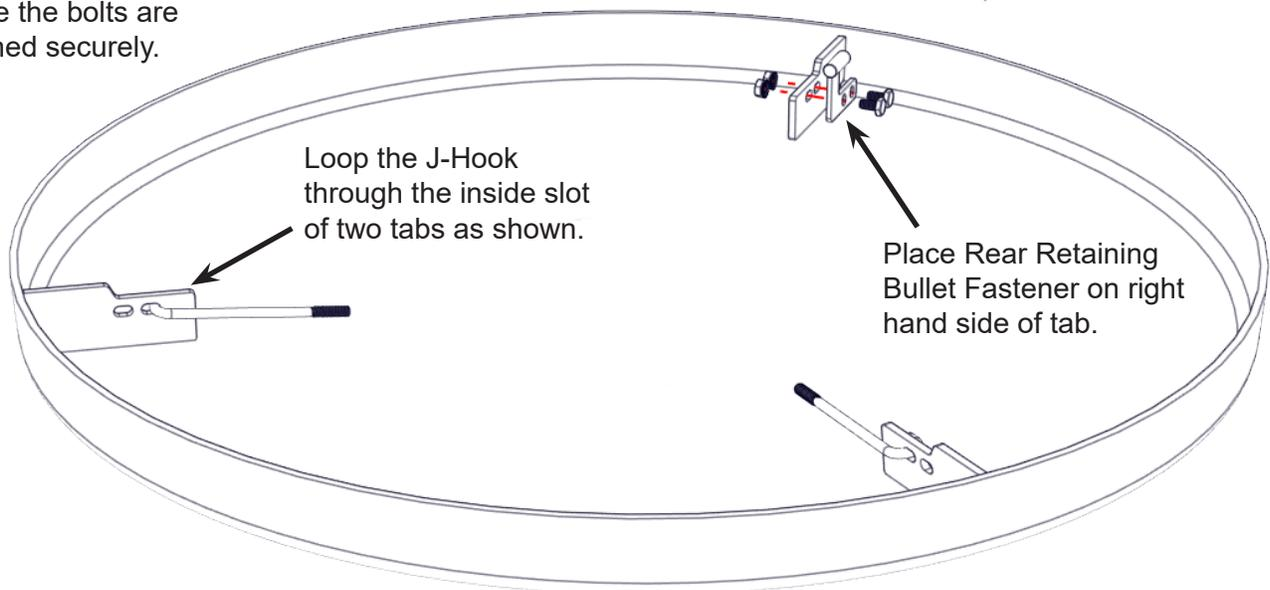
Loop the J-Hook through the inside slot of two tabs as shown.
