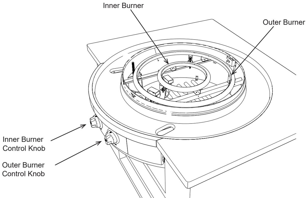
**Inner Burner and Inner Control Knob** - The Inner Burner is a 10" diameter gas fired burner operating at 24,000BTU's. This burner is controlled by the Inner or center-most control knob. Temperatures are adjustable from 225F° to 550F°. Starting at the Off position, the Inner Control Knob rotates 180-degrees counterclockwise through three positions.
