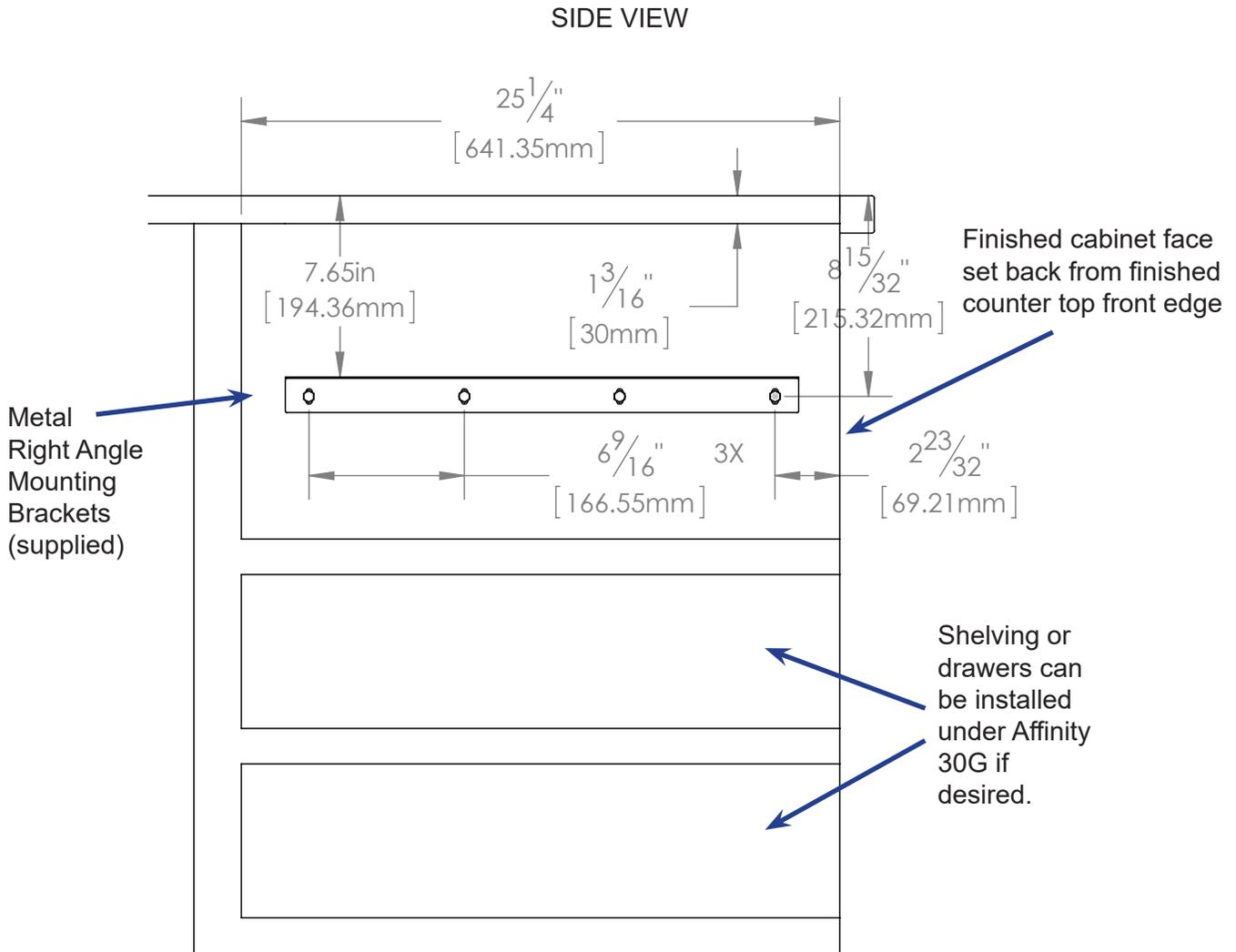
Example of  $\frac{3}{8}$ " tile with substrate for a minimum 3 cm ( $1\frac{1}{5}$ ") overall. Make sure you allow for the counter top overhang as shown.
