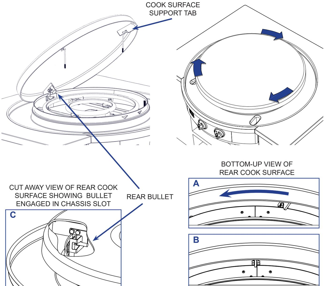
**STEP 9:** Place cook surface over circular skirt with the three support tabs (located under cook surface) resting on the chassis skirt top. Position the rear support tab of the cook surface to the right of the rear seam (rear view) of the chassis skirt (A). Then rotate the cook surface clockwise until the support tab is in line with the seam (B) and the rear bullet secures in the chassis slot (C).
