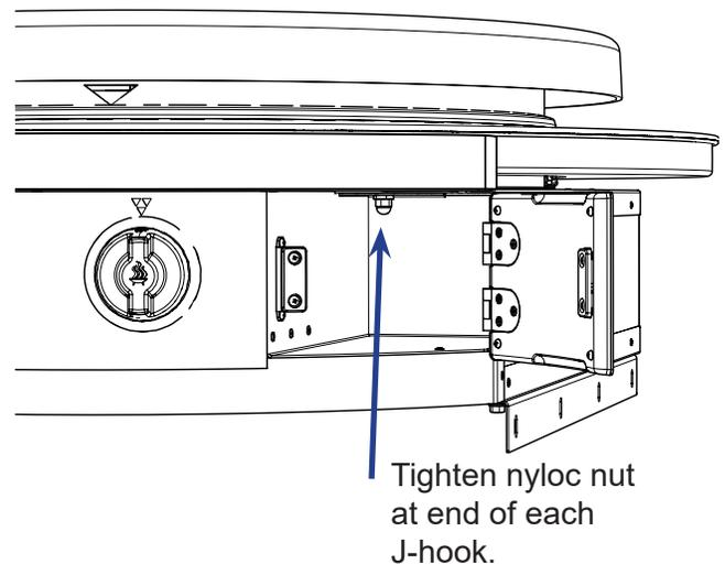
**STEP 10:** Locate two (2) J-hooks attached to underside of cooktop, cut zip ties and remove nyloc nut.
