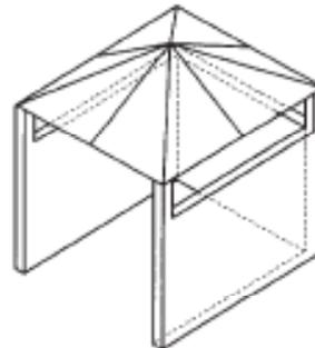
Figure 4 - Open side at least 25% of total wall area. 30% or more of the remaining wall area is open and unrestricted
