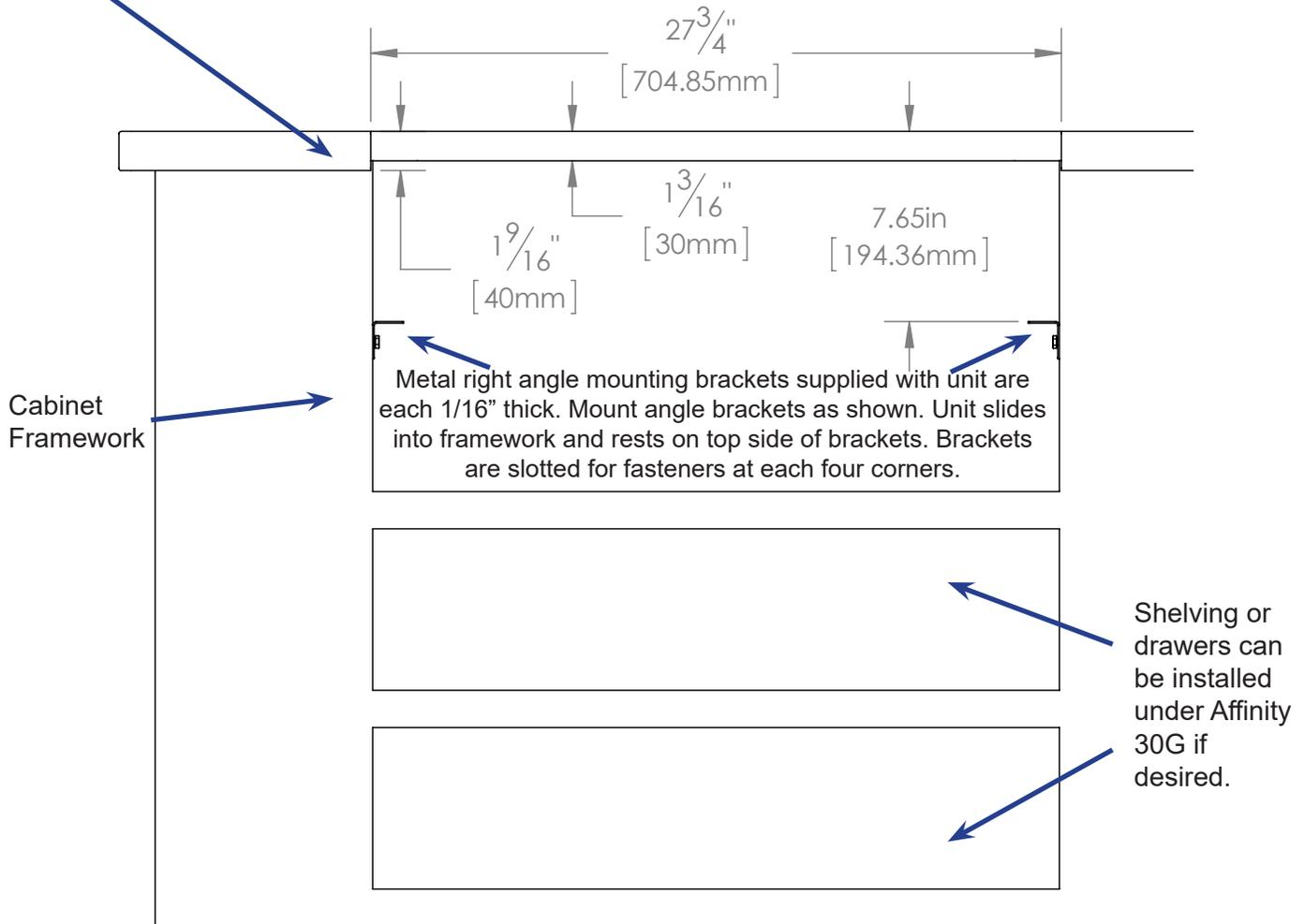
**STEP 3:** Construct a bay for the Evo unit with your chosen cabinet system. Position and fasten the supplied mounting brackets 7.65" below the finished counter top surface.
