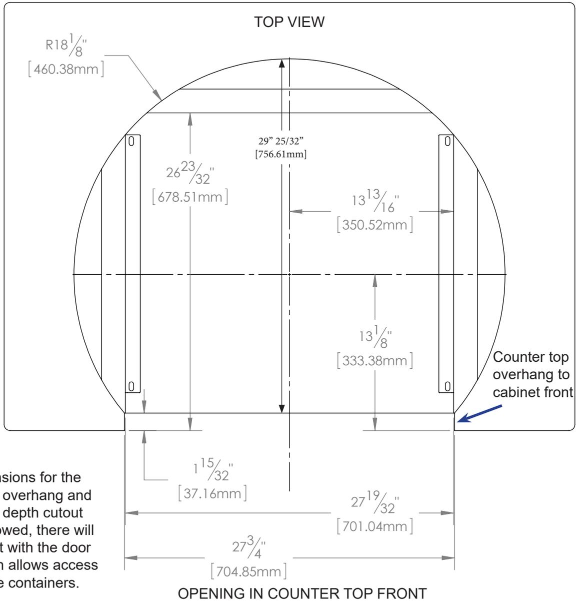
**STEP 2:** Mark the finished position of the Evo Affinity 30G drip pan on the counter top using the dimensions shown. The circular dimension of 36.25" is the diameter of the drip pan to the outside material thickness (e.g. to the inside of the rolled bead edge). The drip pan cutout must be made precisely to these dimensions (or at a maximum +1/16") so that the half-rolled top bead on the drip pan edge overhangs the cutout dimension by .25". (See following page for more details).
