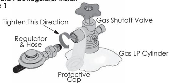
Quick Disconnect Hand-Wheel Regulator Install
